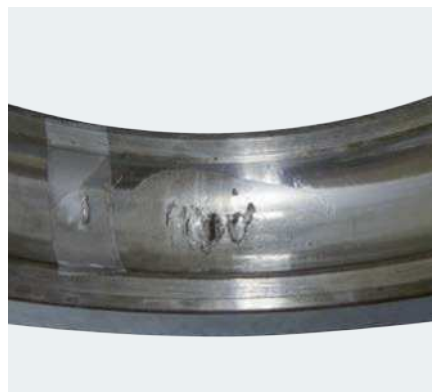
Ball bearing raceway with large spalls due to excessive current erosion
